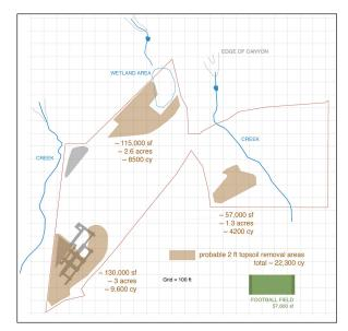
Note that the amount of dirt to be excavated and repositioned on the site is much larger than just the cuts that produce spoils. ~ 2 feet of topsoil must be removed in all areas to receive spoils, stored on the site and then recovered over spoils.
