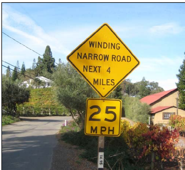
Photo 1: Posted Advisory Speed of 25 MPH just north of Lambert Bridge Road intersection (note posted speed does not establish roadway speed limit)
